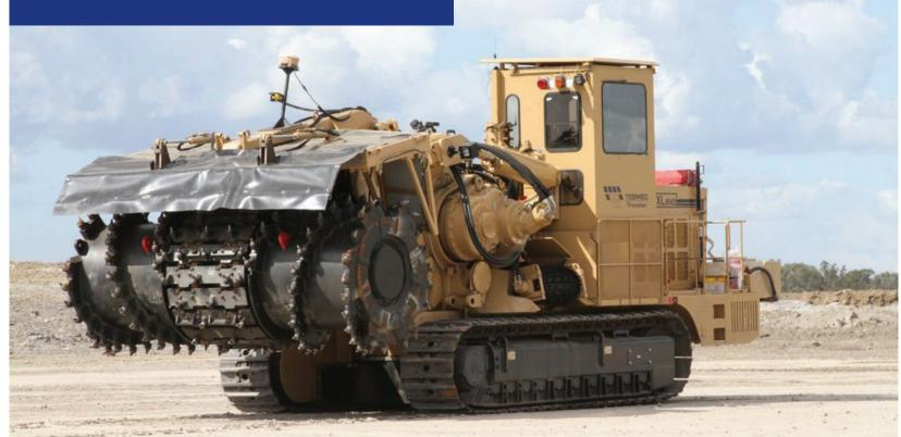
Tesmec 1475XL EVO Rockhawg is a high performance 115 metric ton-class surface miner featuring a 630 HP (470 kW) engine employed in bulk excavation and tunneling projects, surface mining, tunneling and very large diameter pipelines
