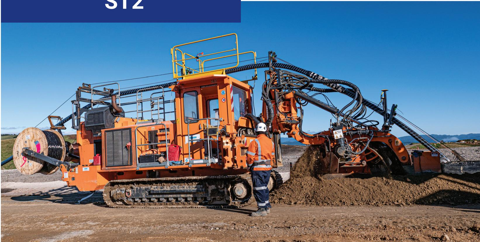
Tesmec ST2 is a 25-30 metric ton-class trencher featuring a 510 HP (375 kW) Tier 4/Stage V engine, or a 536 HP (394 kW) Tier 3 engine, designed to allow the simultaneous trenching and mechanical laying for the deployment of networks in rural environments and rocky grounds
