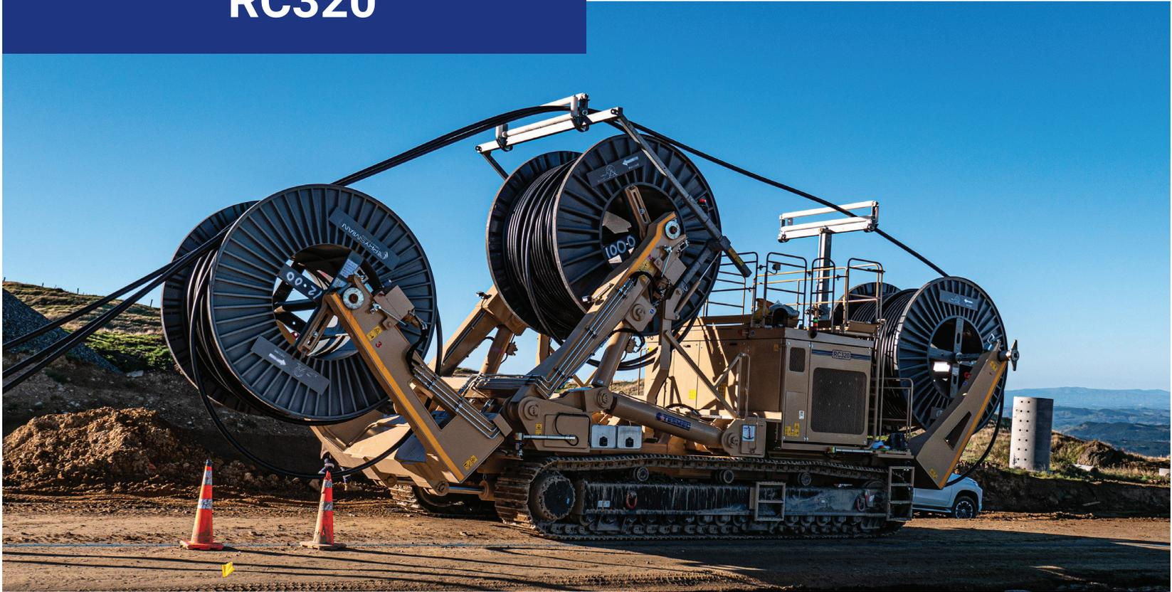
Tesmec RC320 is a 44 metric ton-class reel carrier featuring a 250 Hp (186kW) Tier 3 engine, or a 275 HP (205 kW) tier 4/Stage V designed to carrying and unrolling cables or pipes. It is conceived for energy cable projects.
